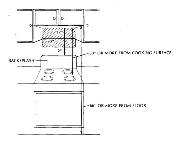
For removal of the Microwave/Hood System bottom cover for cleaning or servicing, a 2-inch space is necessary between the top of the range backsplash and the bottom of the Microwave/Hood System.
